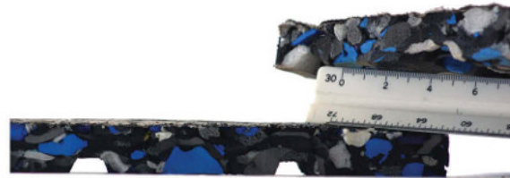
Picture 2. In-plane drainage channels to maximize horizontal flow
